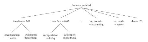
Fig. 3: A portion of a Meta-CLI configuration tree
