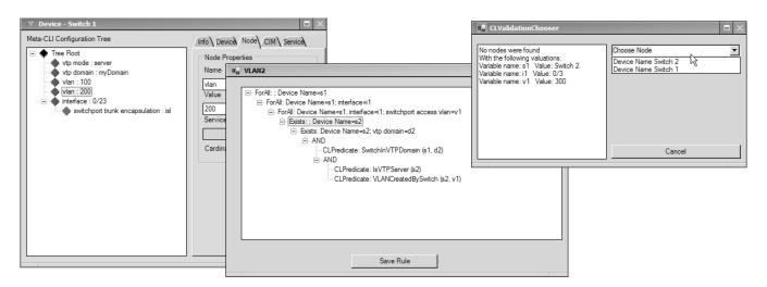
Fig. 4: Illustrates a screenshot from ValidMaker's configuration view. The configuration of a device is abstracted as a tree of name-value pairs (left window). When a CL constraint is violated on a given configuration, ValidMaker highlights the part of the formula that is false (center window). The user is presented a list of tree nodes that violate that part of the formula (right window). The validation can then be resumed on one of these nodes to further explore the cause of the violation.
