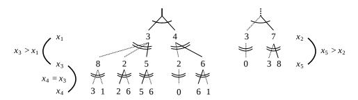
Fig. 6: The and/or tree for the configuration of Figure 5, for the two dependency chains identified earlier. Single arcs indicate conjunctions, and double arcs indicate disjunctions.
