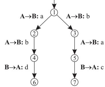
Figure 3. A protocol sensitive to message shuffling
