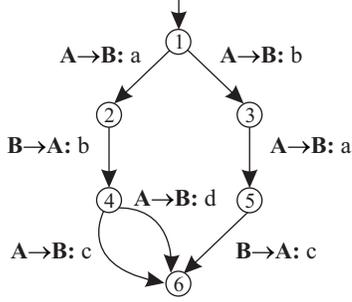
Figure 5. A fixable protocol specification
