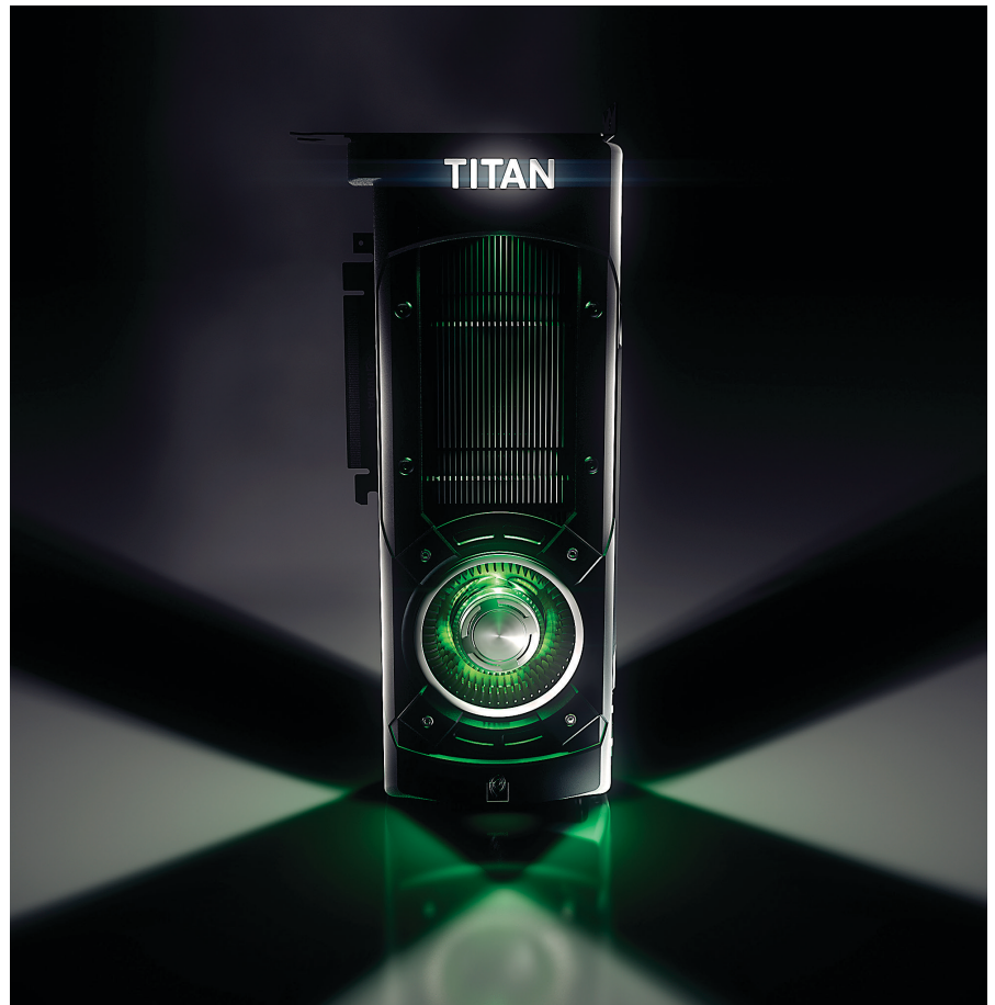
Nvidia's Titan X graphics card, featuring the company's Pascal-powered graphics processing unit driven by 3,584 CUDA cores running at 1.5GHz.
