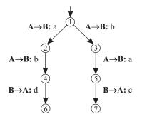
Figure 3. A protocol sensitive to message shuffling
