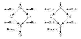
Figure 4. Two simple protocol specifications
