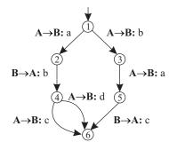
Figure 5. A fixable protocol specification
