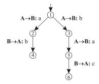
Figure 1. A simple protocol specification
