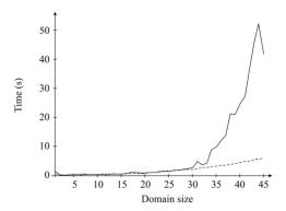
Fig. 2. Validation time (in seconds) for Choreography Specification 1 with respect to the size n of the domain, using respectively the explicit quantification (dashed curve) and the freeze quantification approach (solid curve).
