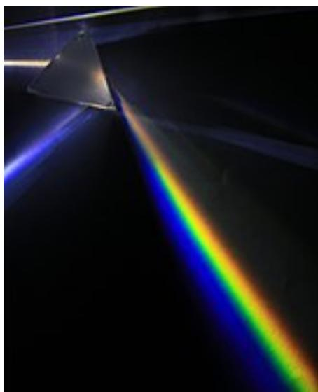
Isaac Newton shone a narrow beam of sunlight through a glass prism, which split the white light into its colours, which he called a spectrum. The colours blend smoothly into each other, but they're generally grouped into six or seven colour names: red, orange, yellow, green, blue, (indigo), violet. Then he passed the coloured light through another prism turned upside down with respect to the one in the picture, and white light came out the other side.
